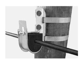
Basic Suspension Hardware ADSS, Lightweight, quick installation, can be installed with through bolt and / or stainless steel strip. The scope of application is: aerial, wall-mounting, pole, Span 200 meters.
